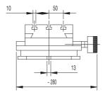
The MG-0 coordinate table provides precise adjustment of the image onto a printed part and is produced from stable cast iron. The MG-0 is especially well-suited for the larger printing machines or for the assembly of heavy tooling fixtures. It allows for adjustments in the x- and y-axes through the use of fine adjustment knobs with a vernier. The w-axis adjustments are carried out using a marked scale.
