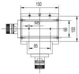
The KT 50 coordinate table is produced from stable cast iron. Due to its solid and yet compact construction, the KT 50 is well-suited for applications requiring critical print image adjustments onto parts with smaller and middle-sized print machines. It is often used on shuttle tables as well. Infinitely variable adjustments can be made in the x- and y-axes using the fine adjustment knobs with a vernier. The w-axis adjustments are carried out using a marked scale.
