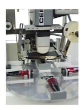
The machine can provide hot stamping on the bottles and jars which have been previously screen printed
