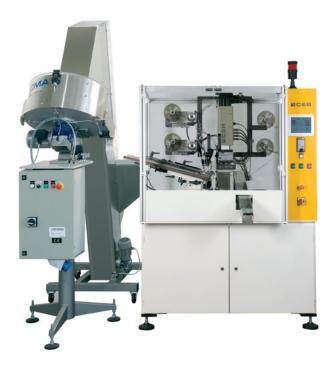
Throughput of up to 4,500 caps per hour for contouring over  $360^{\circ}$
