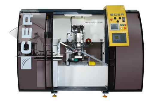
$\label{thm:linear} \mbox{High-throughput machine for hot stamping of industrial counter} \mbox{ wheels.}$
